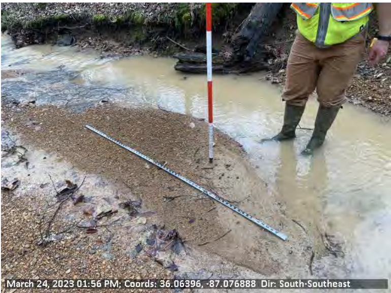
21 View of STR-6-J1 proposed sediment removal locations on left descending bank. First deposit is approximately 8'x3', and 0.5" deep.
