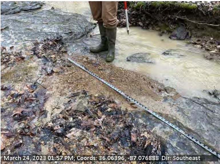
22 View of STR-6-J2 proposed sediment removal location on left descending bank. Second deposit is approximately 3'x2', and 0.5" deep.
