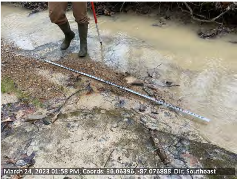
23 View of STR-6-J3 proposed sediment removal location on left descending bank. Third deposit is approximately 4'x1', and 0.5" deep.
