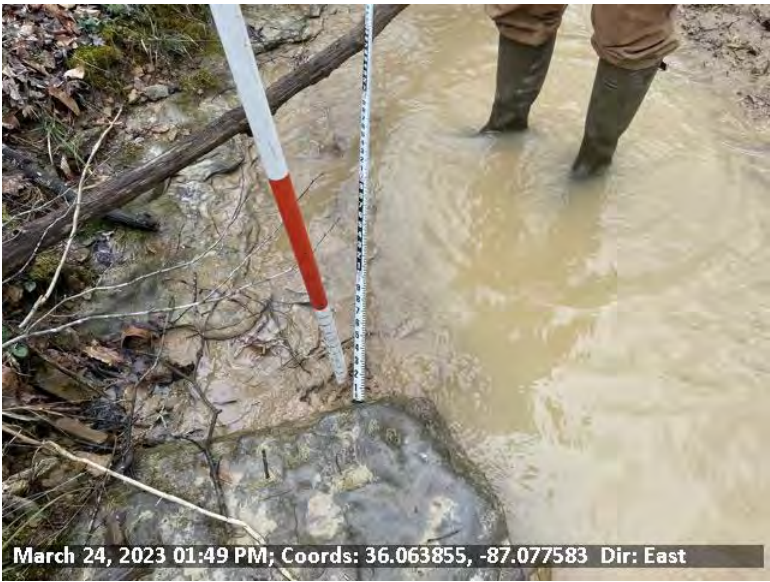
24 View of STR-6-K1 proposed sediment removal location on left descending bank, measuring approximately 2'x1', and 1" deep.
